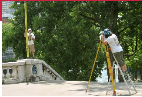
Topometric monitoring of the Viaduct of Passy (Paris) - levelling operations
