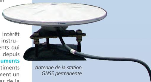
Antenne de la station GNSS permanente
